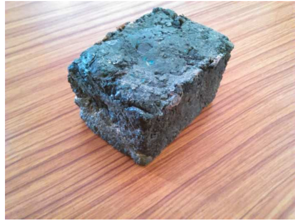
Fig 5.1 Plastic & Slag mix Product with 3.0'x 2.0'x 1.5'
